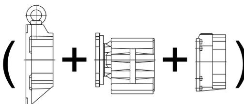
(System cover + Intermediate gear + System cover)
