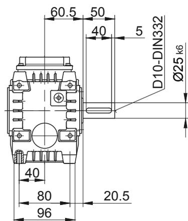
Foot with clearance holes at bottom
