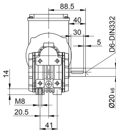
Foot with clearance holes at bottom
