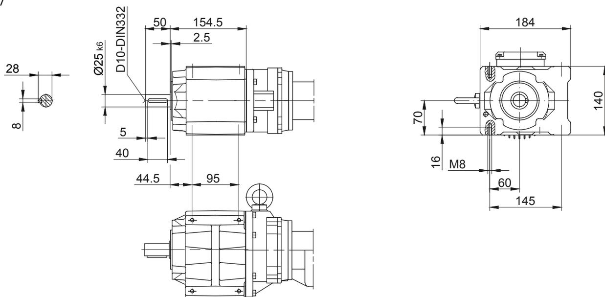
Foot mounting right with clearance holes
