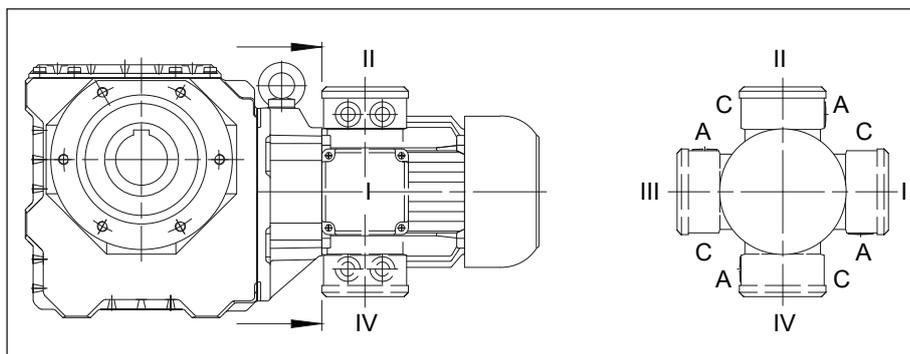
Turning or rotating the gearbox in space in the different mounting positions according to DIN 42950 does not influence the marking as shown. The details of the terminal box always show the position of the terminal box and the cable entry in relation to the gearbox and not in space. The mounting according to DIN 42950 is to be given separately.
