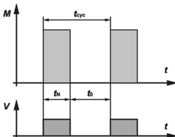
S3 duty consists of a sequence of identical cycles, each composed of an operating time with constant load and a rest time with the windings de-energised. The cycle is such that the starting current does not significantly affect the temperature rise. The operating time under rated load and the subsequent pause are both short. The equipment can operate under load only during the period indicated by the duty cycle as a percentage of the total cycle time (cycle duration).
