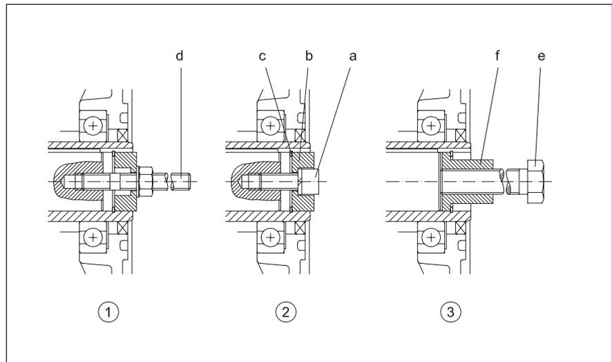
Detailed information on shaft-mounted gear units, bevel-gear units and worm-gear units is available (see chapter 11, 12., 13 dimensional drawings "Tools for fitting shaft-mounted gear with hollow shaft and keyway").
