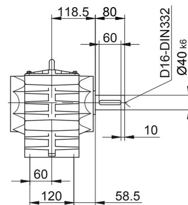
Foot with clearance holes at bottom
