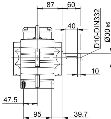
Foot with clearance holes at bottom
