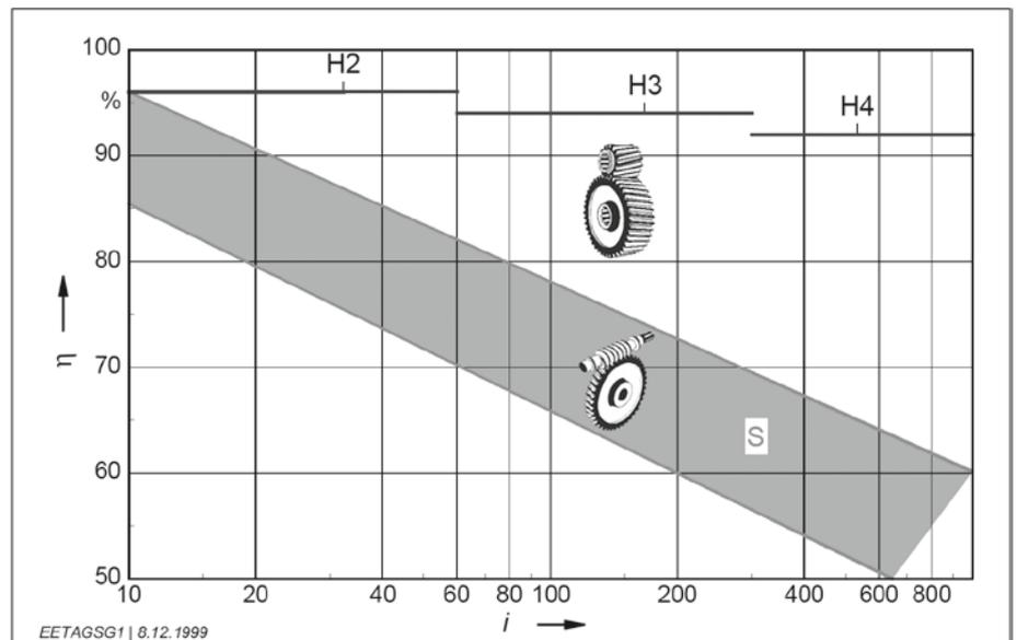
Comparison of typical efficiency ( $\eta$ ) versus reduction ratio ( $i$ ) for helical spur gear units (H) with two, three or four stages and two-stage worm gear units (S), relative to the rated power of the gear unit.
