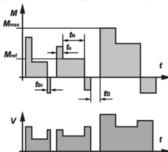
In S9 duty the load and the speed vary non-periodically within the permissible operating range. This includes frequently applied overloads, which must never exceed the reference load. For this duty type, a constant load appropriately selected and based on duty type S1 shall be taken as the reference value  $M_{ref}$  for the overload.
