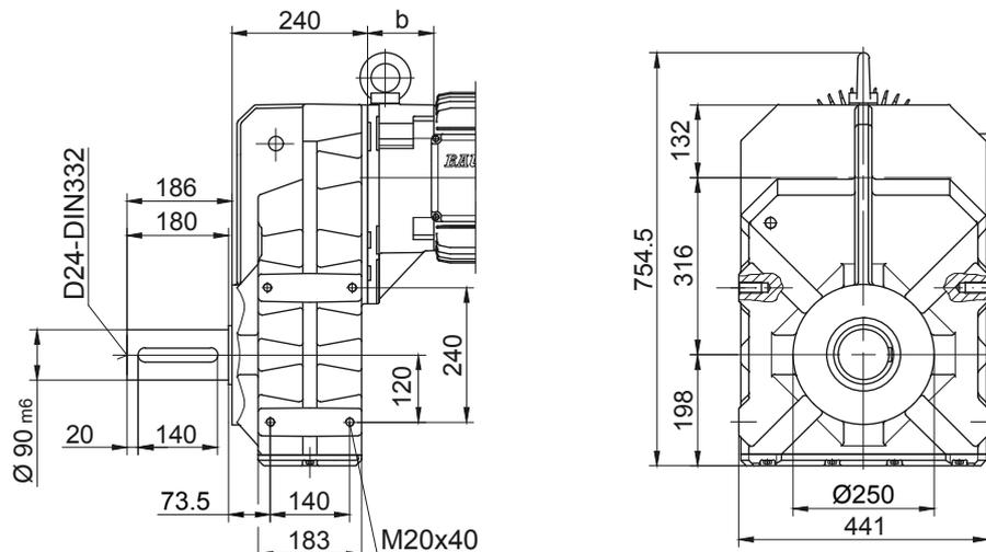
The actual gearbox design can vary from the geometry shown. Generate drive specific 3D and 2D geometries under [www.BauerCat.com](http://www.BauerCat.com).
