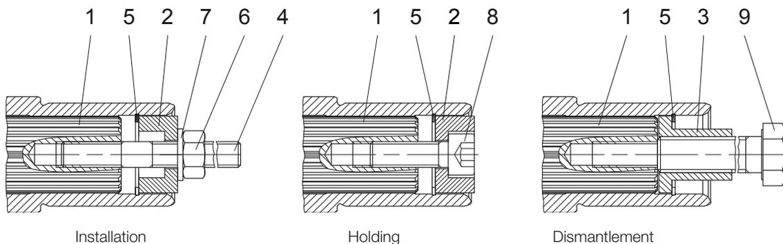
The parts shown are necessary for assembly. ONLY \* specified parts are enclosed in the assembly kit. Suitable measures are to be used to secure Bolt Pos. 8 against loosening!
