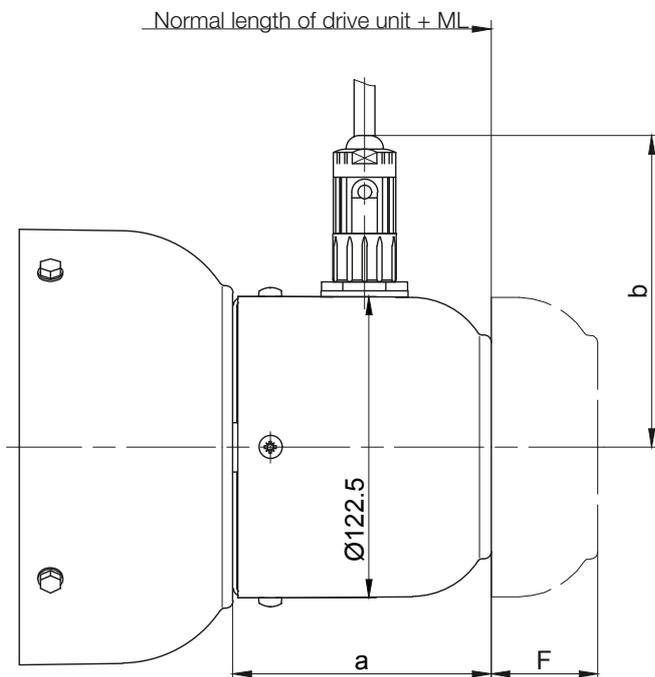
Fan cover geometry for D..16 and D..22, see dimensional drawing: terminal box as standard version
