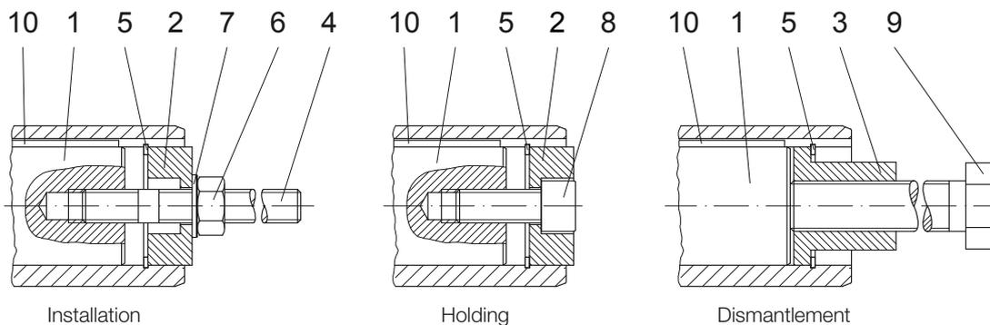
The parts shown are necessary for assembly. ONLY \* specified parts are enclosed in the assembly kit. Suitable measures are to be used to secure Bolt Pos. 8 against loosening!
