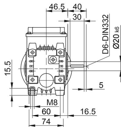
Foot with clearance holes at bottom
