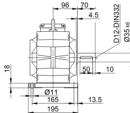
The actual gearbox design can vary from the geometry shown. Generate drive specific 3D and 2D geometries under [www.BauerCat.com](http://www.BauerCat.com).
