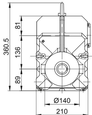
The actual gearbox design can vary from the geometry shown. Generate drive specific 3D and 2D geometries under [www.BauerCat.com](http://www.BauerCat.com).
