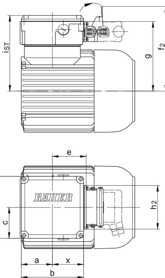
Fan cover geometry for D..16 and D..18, see dimensional drawing: terminal box as standard version
