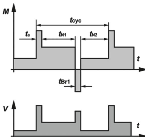
The machine runs continuously under variable load with frequent speed variations. The machine can operate continuously in this manner if at each speed the specified values are not exceeded (moments of inertia  $J_M$  and  $J_{Ext}$  cycle duration (if other than 10 minutes), rated output and duty cycle. With a moment of inertia of  $1 \text{ kg m}^2$ , the acceleration characteristics are the same as with a mass of  $1 \text{ kg}$  at a distance of  $1 \text{ m}$  from the axis of rotation).
