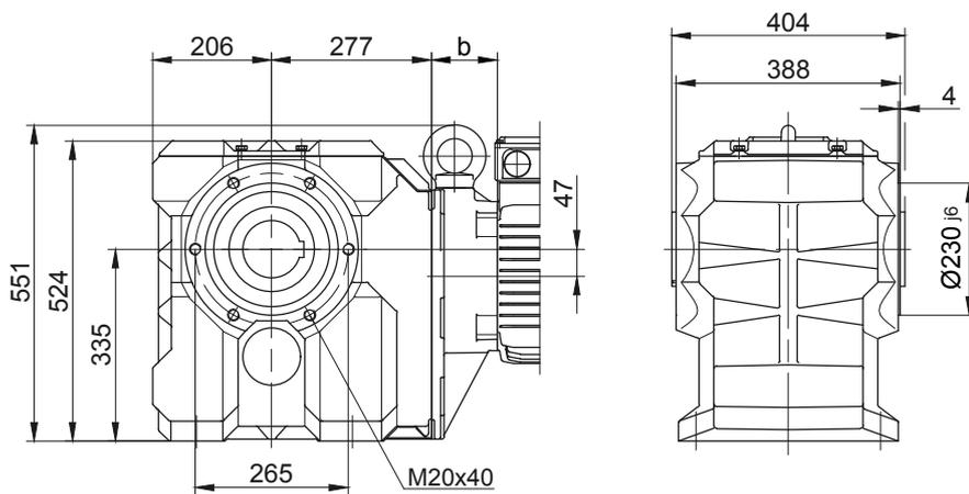
Foot with clearance holes at bottom
