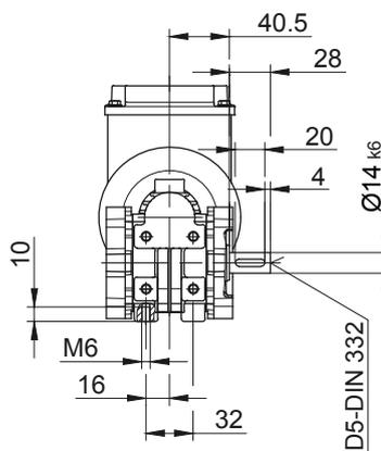
Foot with clearance holes at bottom
