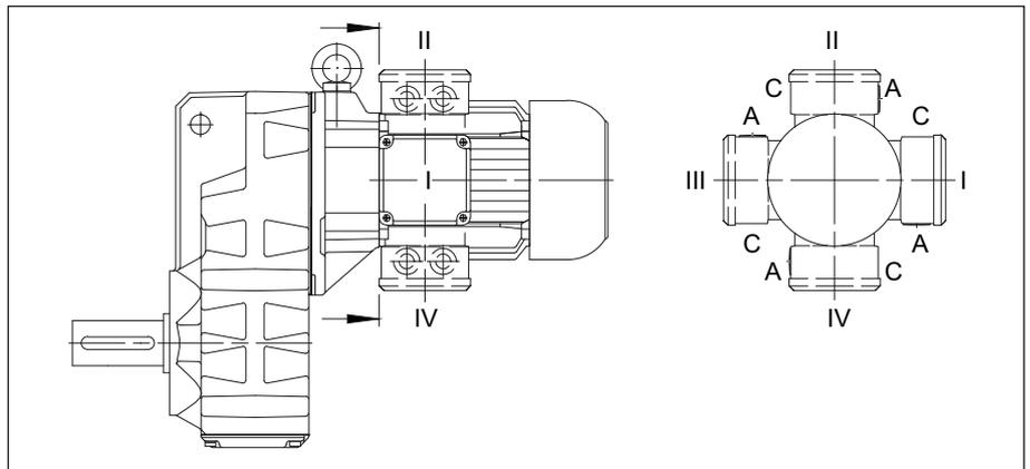
Turning or rotating the gearbox in space in the different mounting positions according to DIN 42950 does not influence the marking as shown. The details of the terminal box always show the position of the terminal box and the cable entry in relation to the gearbox and not in space. The mounting according to DIN 42950 is to be given separately.
