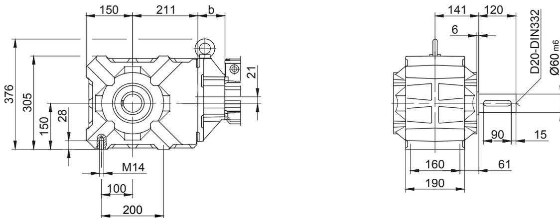
Foot with clearance holes at bottom
