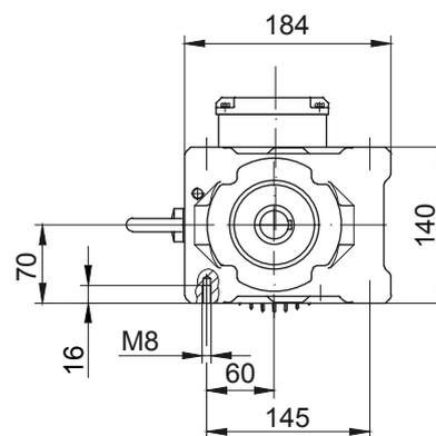
Foot mounting right with clearance holes
