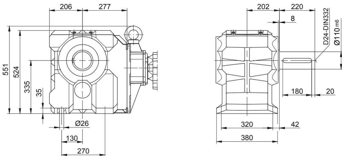
The actual gearbox design can vary from the geometry shown. Generate drive specific 3D and 2D geometries under [www.BauerCat.com](http://www.BauerCat.com).
