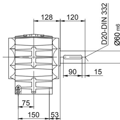
Foot with clearance holes at bottom
