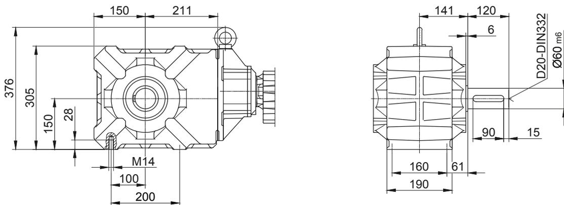
Foot with clearance holes at bottom
