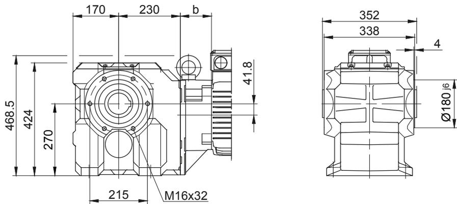
Foot with clearance holes at bottom
