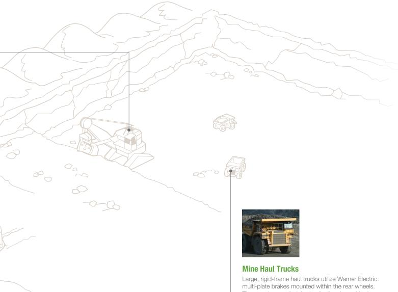
These spring-applied, hydraulically-released brakes are sealed and oil-cooled. The axles are connected to the transmission using power-dense U-joints.
