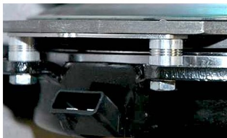
Very simple, no hassle re-gap option is a standard feature which doubles clutch life.
