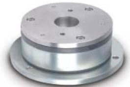
Varistop achieves this with variable torque braking, offering smooth operation with stepless torque change. Electric current that produces torque can be electronically controlled and varied depending on the weight of the load and height at which it is carried. This allows the truck to be braked from speed to rest as quickly as possible without becoming unstable.
