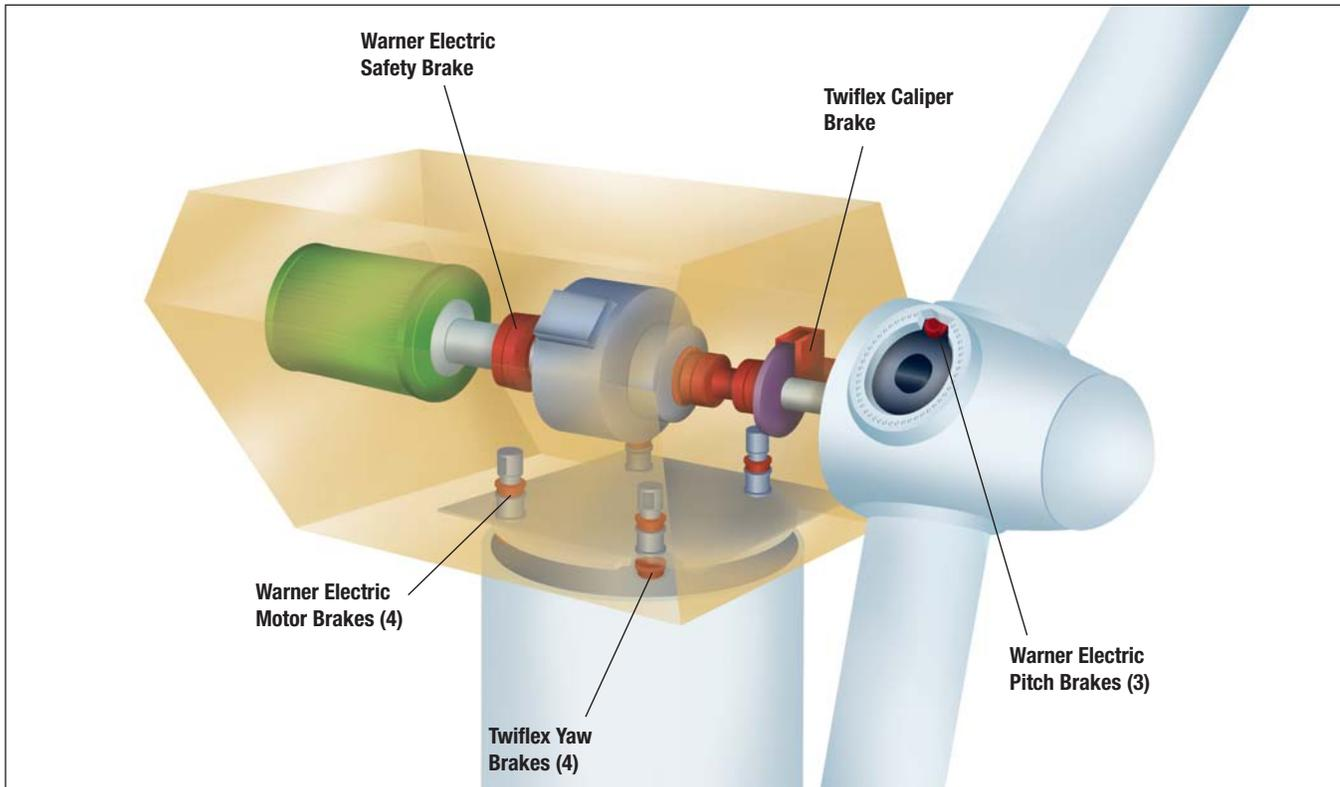
These requirements are more difficult to meet on the high-speed shaft because speed and space will be limiting factors with regard to the maximum disc diameter and brake selections. Nevertheless, high-speed shaft braking has been used on many turbines rated up to 750 kW, although as the industry develops higher capacity turbines, the trend is leaning towards rotor-shaft braking.
