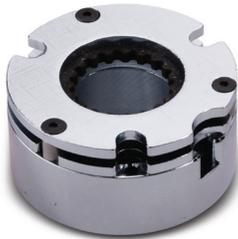
Matrix spring-applied, electromagnetically-released 1EB Series servo motor brakes are widely used on industrial robot applications. The brakes maintain torque during static/holding operations and occasional E-stop (dynamic stopping) engagement in the case of power failure.
