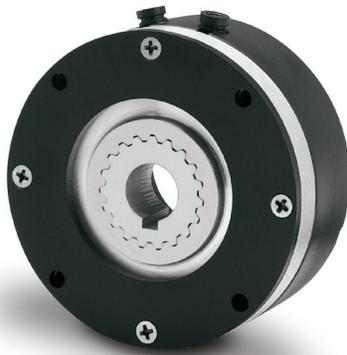
Warner Electric ERS Series brakes are springset and electrically-released to provide holding as well as occasional dynamic stopping functions in emergency situations.
