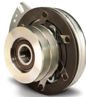
Warner Electric engineers developed a modified CMS (Commercial Mag Stop) clutch to meet a pump jack OEMs function and performance requirements. The clutch assembly mounts directly to the engine shaft and features a double-groove pulley to accommodate twin V-belts that drive the pump shaft.
