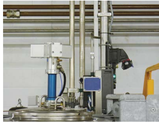
Huco Dynatork piston air motors are often installed on auto paint lines. The air motors are mounted to the top of paint drum agitators ensuring constant rpm of the agitator blade. The result is a better surface finish, lower running costs, and quieter operation.
