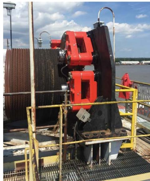
The braking upgrade allowed the use of the existing brake mounting pedestals saving an estimated \$60,000 compared with the costs of completely replacing the system.
