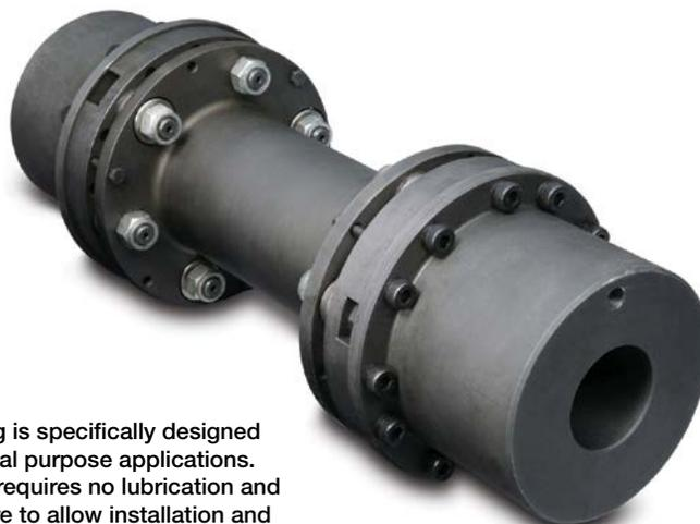
TB Wood's Torsiflex coupling is specifically designed for process pump and general purpose applications. This all-metal disc coupling requires no lubrication and incorporates a plug-in feature to allow installation and removal without disturbing the pump alignment.
