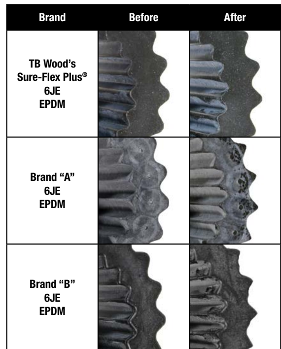
Figure 7: Tooth shape, before and after 450-hour wear test, 6JE TB Wood’s Sure-Flex Plus coupling vs. competition
