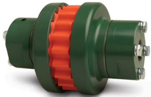
5-Piece TB Wood's Sure-Flex Plus® conventional spacer couplings are designed for easy replacement. The entire center section of the coupling (two flanges and sleeve) can be dropped out by simply removing the flange-to-hub bolts.
