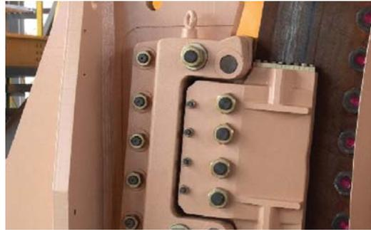
Figure 8: VMS-DP Caliper Assembly (showing reactive backplate)
