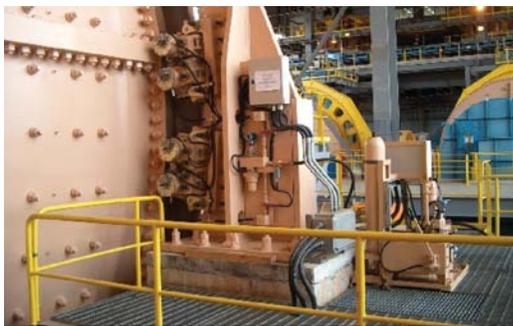
Figure 2: Sossiego Mill Braking System
