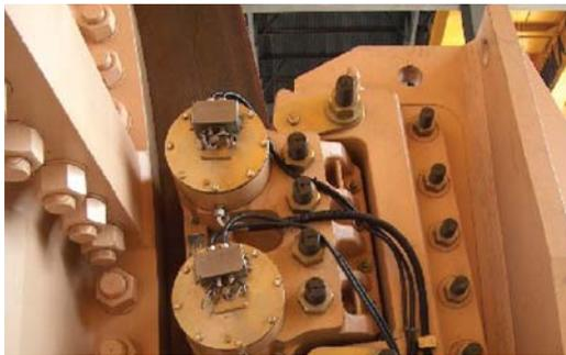
Figure 7: VMS-DP Caliper Assembly (showing spring module)
