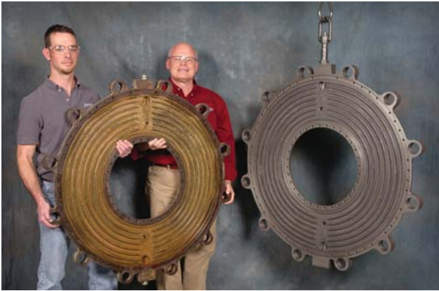
A new 36" composite water jacket (left) weighs approx. 95 lbs. A comparable 36" cast iron jacket (right) weighs approx. 375 lbs. The reduced weight is a significant maintenance benefit, especially when units are installed in weight restricted applications such as mobile yarders in the forestry industry.
