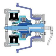
**Stromag KHA** with flexible Periflex® VN couplings for drives particularly subject to torsional vibrations. Connection for SAE flywheels. Housings for SAE sizes 1 to 4 possible.
