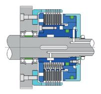
**Stromag KMK** for use in gearboxes (wet operation) with optional disc oil flushing. Hydraulic and cooling oil supplied via the transmission shaft.
