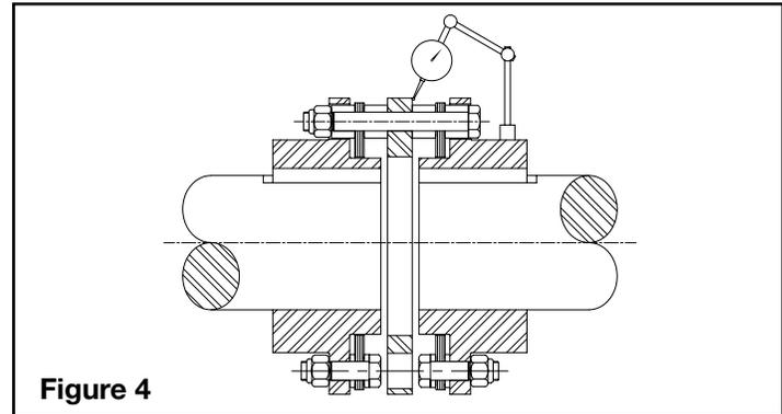
Notes: When the equipment is properly aligned, it is advisable to dowel a right angle gear box to its base. Experience has shown that right angle gear boxes tend to creep in a counter rotational direction. Recheck alignment after doweling.
