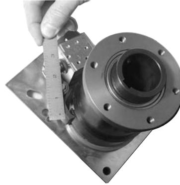
4. The clutch spring should come to rest between two slots. Unwrap the spring and push it backwards into the nearest slot.
