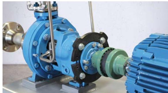
*A size 7 TB Woods Sure-Flex Plus coupling was able to be installed instead of a larger size 8 coupling on this small ANSI pump unit. By utilizing the smaller coupling, the overall package length was reduced allowing for a smaller baseplate footprint.*
